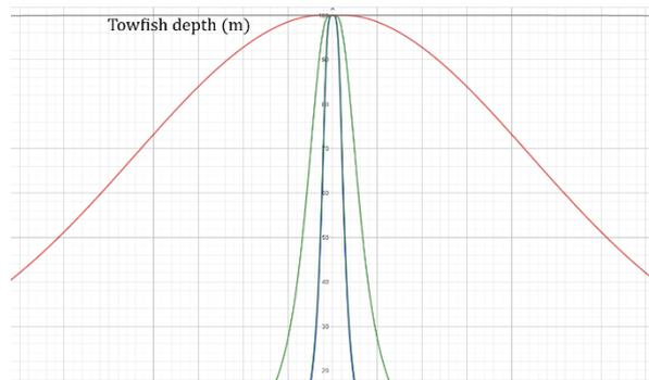
Figure 10 Plot of the function  $D(v)$  in blue and  $f(v)$  with different wire radii (Radius 0.01m: Green line, Radius 0.1m: Red line, Radius 1m: Grey line)
