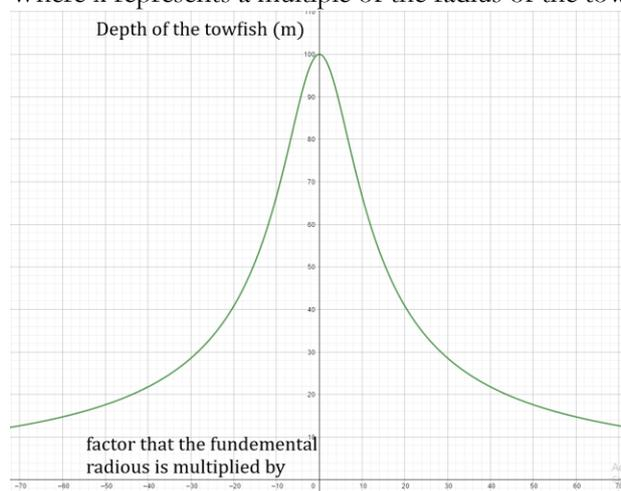
Figure 12 Plot of f(x) showing how multiplying the radius at any point of the towfish by x effects the depth of the towfish
