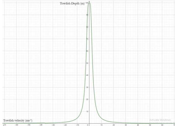
Figure 8 Plot of function  $f(v)$  showing the depth of the towfish when tethered to a real wire plotted against its velocity
