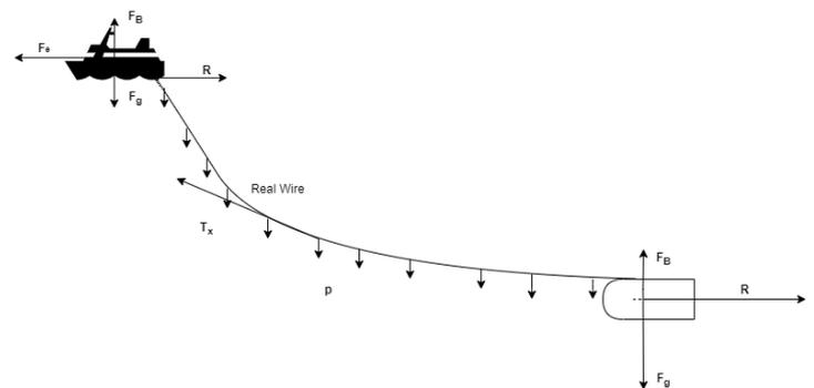
Figure 6 free body diagram showing the vectors acting on the towfish system when the towfish is tethered to a real wire
