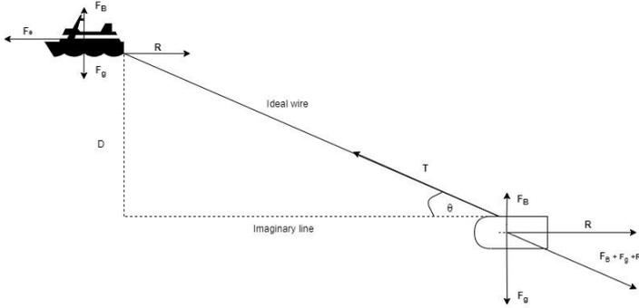
Figure 4 Sketch showing the theoretical triangle formed between the wire and the axes
