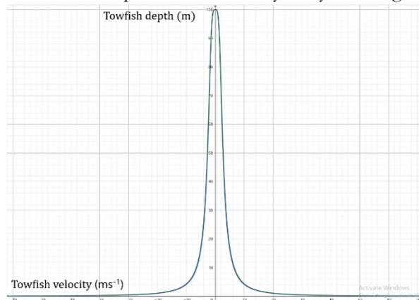
Figure 9 plot of function  $f(v)$  with a wire of radius 0.001 m and  $D(v)$
