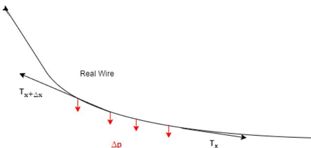
Figure 7 Free body diagram showing how  $\vec{p}$  changes between 2 points in the wire
