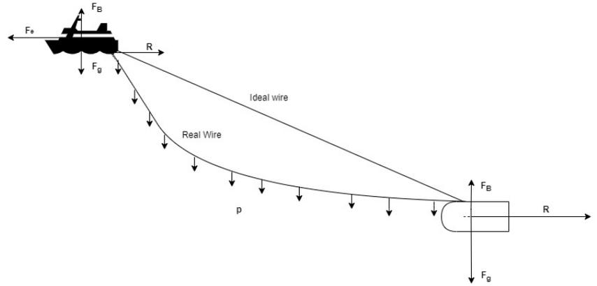
Figure 2 free body diagram showing all the forces acting on the system. where vectors are presented in bold
