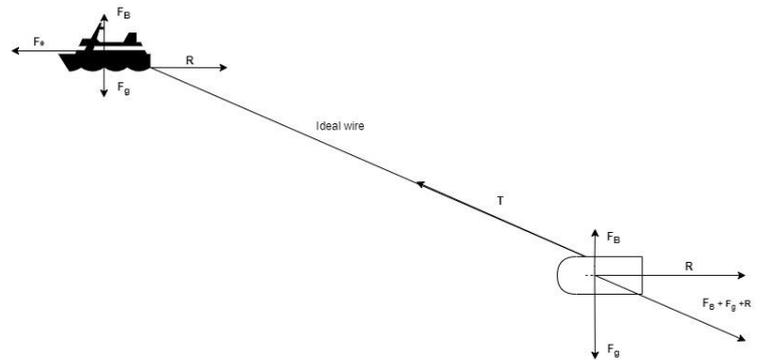
Figure 3 Free body diagram showing vector forces acting on the idealized system
