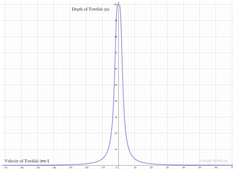
Figure 5 Plot of function  $D(v)$  showing the depth of the towfish plotted against its velocity
