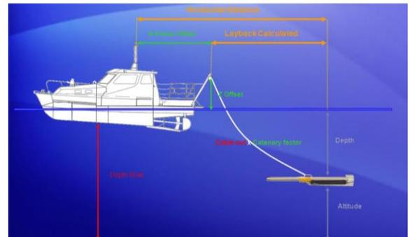
Figure 1 Schematic showing a towfish vessel system (Townsend)
